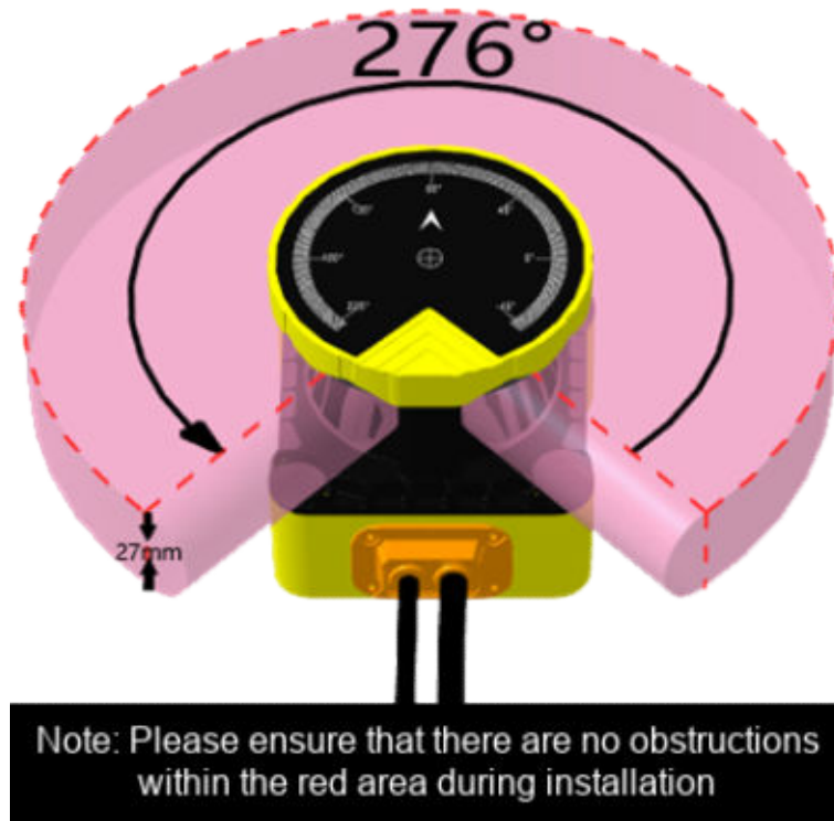
Figure 8 Scanning range Schematic Figure
